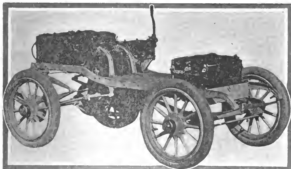
Fig. 3—Model 17 chassis, showing battery in front and rear, motor suspended from yokes, means of adjusting chains, and shaft drive
